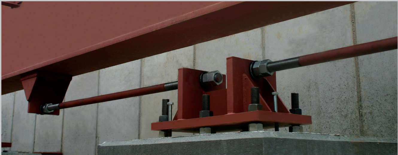
With rigid checking, the A.A.R. rail scale platform remains stable. This stability reduces component wear and the time necessary to capture accurate weightment data.
