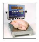
The NexWeigh's GORE-TEXTM vent keeps water out, while allowing pressure and gasses inside the instrument to escape.
