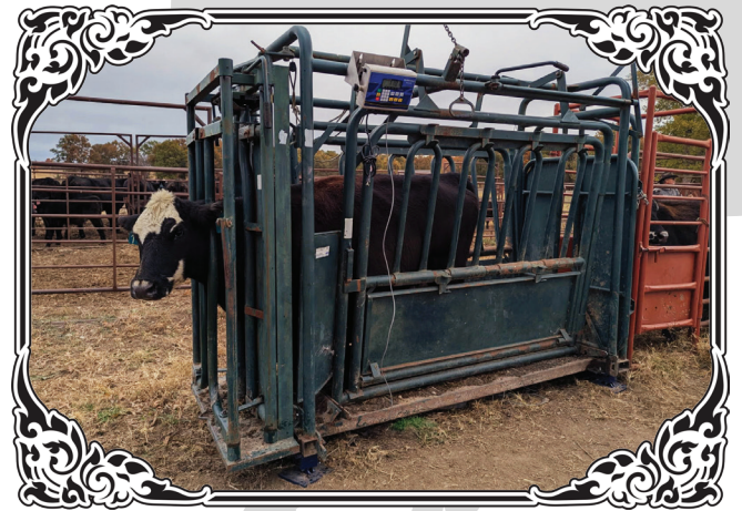
THE LIVESTOCK SCALE BARS IN THE FIELD CONNECTED TO A FAIRBANKS' FB2255 INSTRUMENT.
