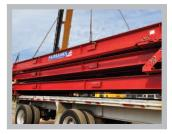
Scale is delivered. anchored, wired to instrument, calibrated, and approaches installed or formed all in a single day.
