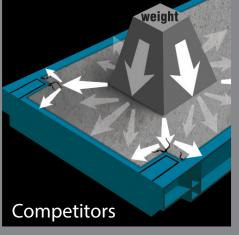
By placing the load cells in easily accessible and serviceable areas beneath the scale, instead of inside the deck, Fairbanks has eliminated the need for cover plates. This design ensures a more structurally sound scale deck that resists metal fatigue, deflection, and internal deck cracks.
