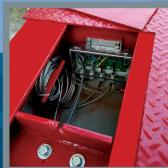
Load cells and electronics are housed in dedicated corner pockets and accessed through easy-to-remove deck plate covers.
