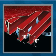
**Competitors'** sealed rib panels can form fatigue cracks in the welds, allowing condensation and rust on the <u>unpainted</u> inside of the supports.
