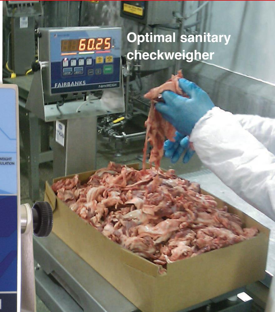
While the NexWeigh is versatile enough for use in a variety of applications, it is ultimately a premium checkweighing instrument due to its sanitary design, commercial approval, IP69K washdown rating and easy-to-use front panel checkweighing functions.
