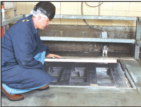
Although one of the heaviest structural steel floor scales in its class, the Lift Deck platform is easily raised and lowered by a single operator for routine cleaning.
