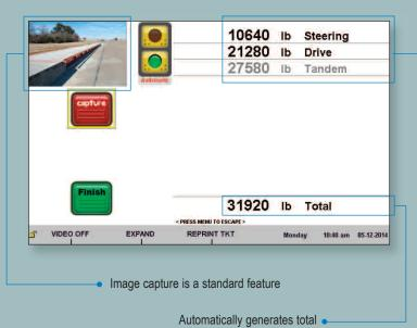
Captures up to 10 axles or tandem axles
