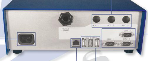
All three FB6000 enclosure styles feature the interfaces and ports shown on the desktop model.
