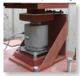
cell movement and premature wear, impact the reliability and accuracy of your scale. Fairbanks has overcome these challenges with massive multi-column load cells integrated into a unique flexural mounting assembly.
