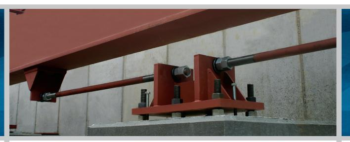
With rigid checking, the A.A.R. Combo scale platform remains stable. This stability reduces component wear and the time necessary to capture accurate weighment data.
