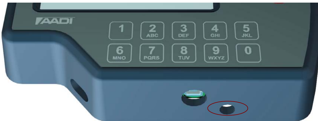
Figure 1-1 The Calibration Switch is placed underneath the Main Unit.
