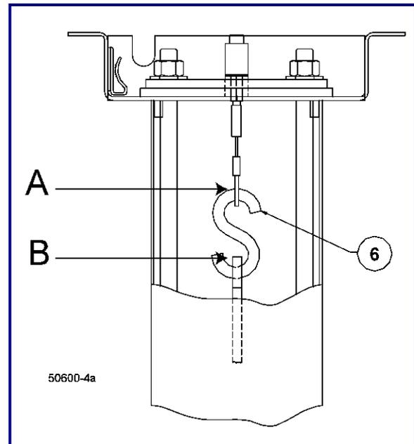
**NOTE:** The lower-end of the **Beam Load Rod Assembly** must be properly hooked into the **Transverse Lever Pivot**.
