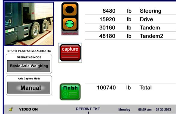
**AUTOMATIC AXLE Capture Mode** *does NOT require* a scale operator if no Product IDs, Customer IDs or other prompts are used in the cycle of operation.
