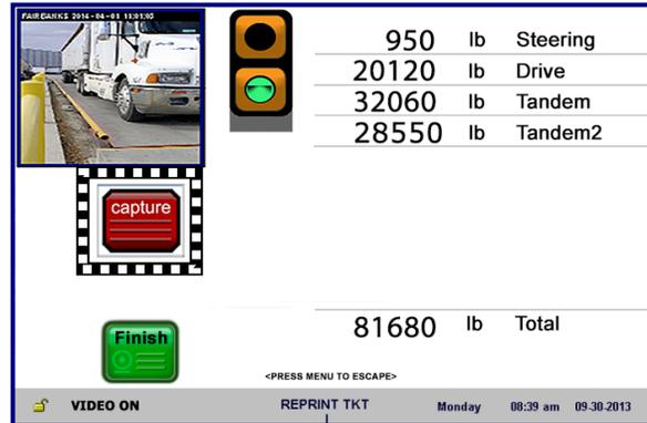
7. Once the axle is into place, the Operator will push the **CAPTURE** button.
