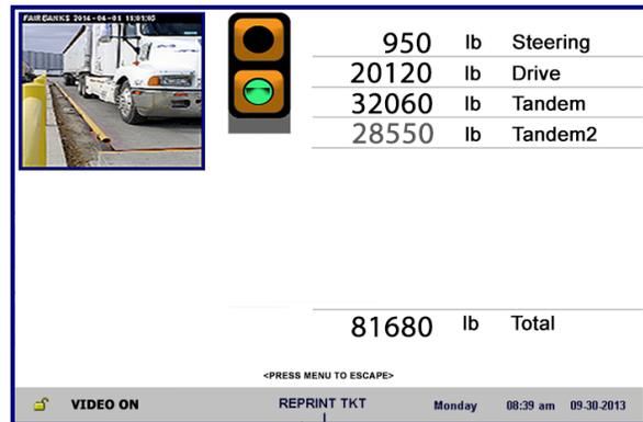
5. Once the system no longer senses additional axles and the total timer has expired, the system will automatic totalize all the captured axle weights.
