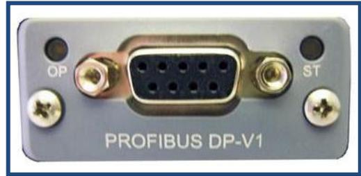
**PROFIBUS-DP** utilizes a **non-powered two-wire (RS-485) Network**.
