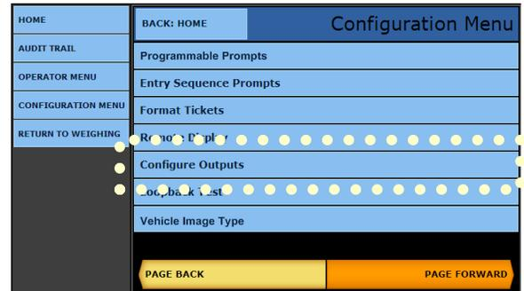
6. Touch the screen to select **CONFIGURE COM X**, where **X** is the desired COM port location to configure the output data string.
