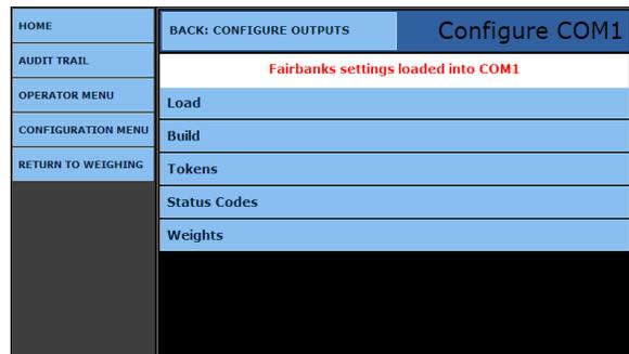
12. Verify the **CONFIGURATION BAUD, PARITY, STOP BITS** to be at the correct values.
