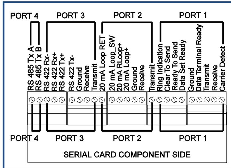
The **SERIAL CARD (30921)** provides **four (4) outputs** with a maximum of **two (2) cards** per Instrument. See the Port Assignments listed below.
