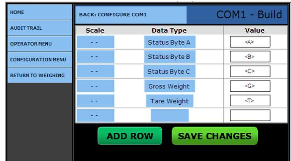
11. Touch the screen under **SCALE** to select the scale where the data item is obtained.
