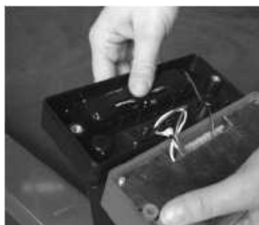
Click the battery holder back into place
