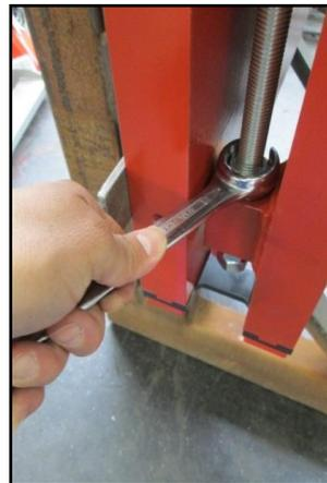
3. Loosen the lower nuts of the tensioning assemblies as well.
