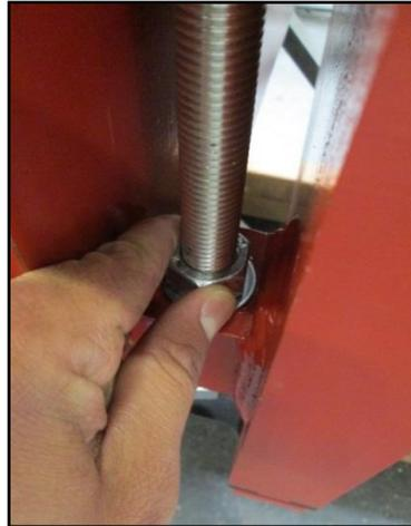
5. Tighten and lock down the lower nuts with a wrench
