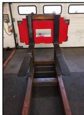
13. Install each fork by aligning it with the cut-out on the bottom center of the weigh carriage front plate then slide each fork to its permanent position.
