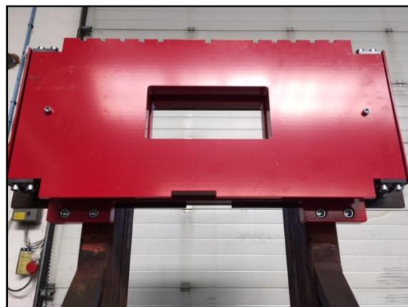
12. Install each fork by aligning it with the cut-out on the bottom center of the weigh carriage front plate then slide each fork to its permanent position.
