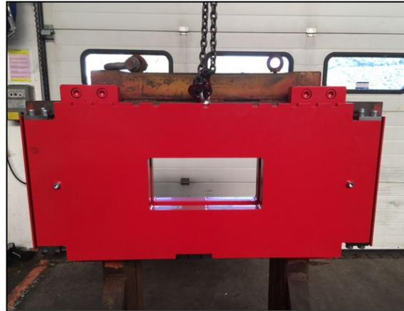
9. Once the upper claws are attached to the original forklift carriage, proceed with installing the lower blocks (lock blocks) on the lower side of the weigh carriage back plate. Torque to 222 foot pounds for 5,000 lb capacity or 443 foot pounds for 10,000 lb capacity.
