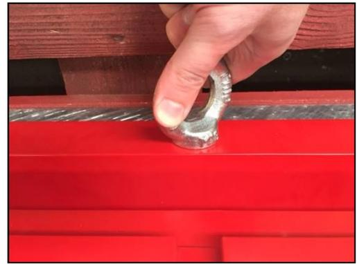
8. Use a properly rated chain/strap to attach to the eye bolt installed in Step 7. and slowly lift the weigh carriage and align with the center of the original forklift carriage. Position the weigh carriage onto the forklift.
