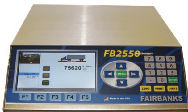
The Desktop FB2550 Instrument has three (3) fully programmable RS-232 DB9 Serial COM Ports, three (3) USB Ports, a VGA and an Ethernet Port.
