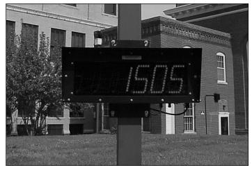
Fairbanks' remote display can be used in applications where a weight display from a distance is necessary — offering a comfortable viewing range up to 160 feet away on the 5.5" model.
